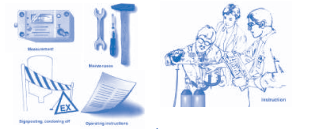
Figure 4.1. Examples of organisational explosion protection measures (12)
