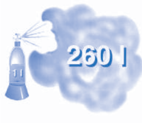
Figure 2.4. Evaporation of even small quantities of flammable liquids (such as liquefied propane) may give rise to large quantities of flammable vapours
