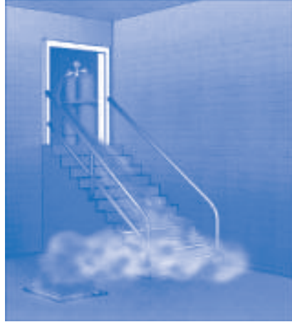
Figure 2.3. Spread of liquefied gases (example) (6)
